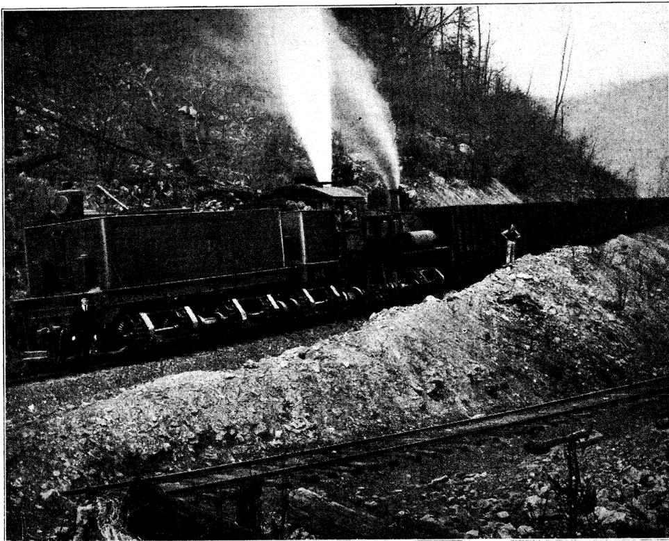
SWITCH BACK.  $4\frac{1}{2}\%$  GRADE, LOOP CREEK BRANCH, C. AND O. RY.
